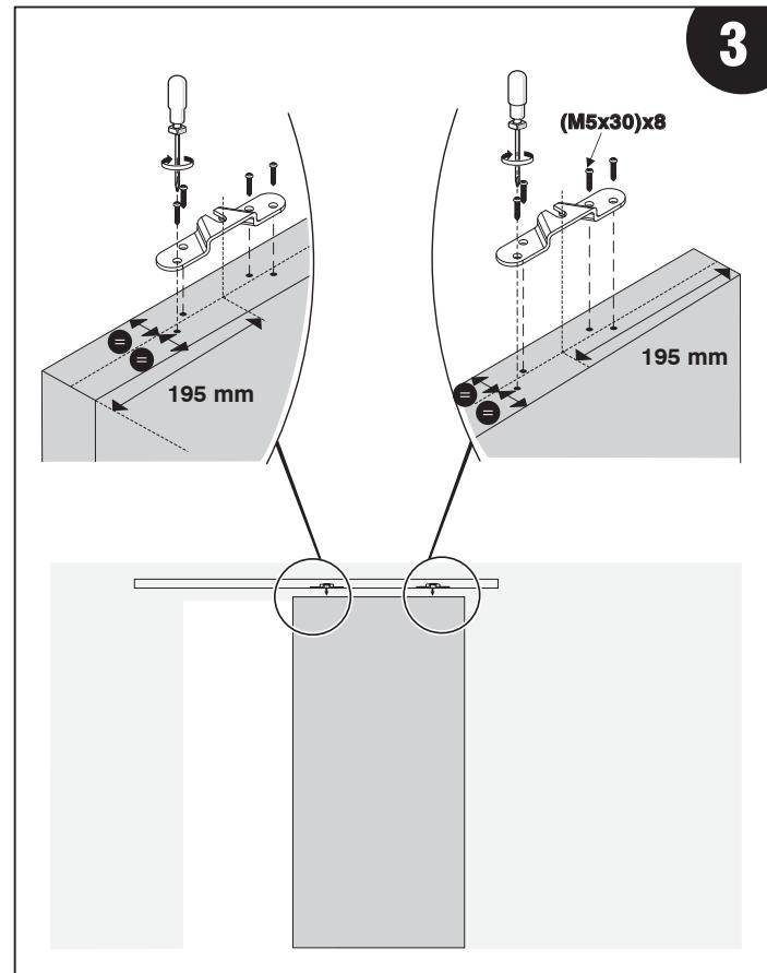
**Step 3: Installing the mounting plates**
