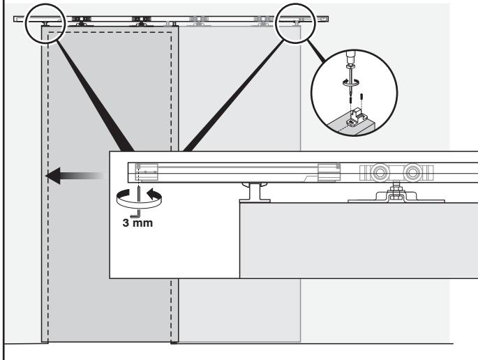
**Step 8: Assembly of the second soft-close damper system and activator**
