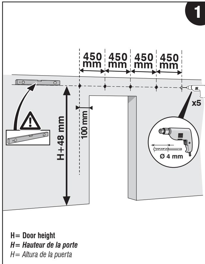
**Step 1: Drilling the wall**
