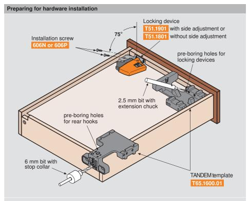
NOTE: Use of the T65.1600.01 TANDEM template is essential for accurate location and angle of pre-bored locking device holes and accurate boring for rear hook holes
