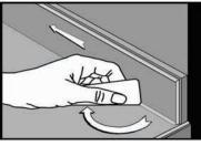
3.) Place longest beveled edge of the PERFECT BEAD TOOL on the horizontal surface and rotate small tip in direction of excess silicone removal.
