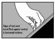
4.) Tilt the PERFECT BEAD TOOL towards vertical splash surface until short beveled edge touches vertical splash surface.
