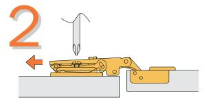
An  $\mbox{\ensuremath{^{\text{\tiny KL}}}}\xspace$  value of 0,7 mm between door and cabinet side is achieved on final assembly.
