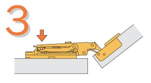
To remove the hinge from the mounting plate, press gently in the places shown by the arrows.
