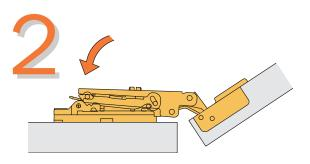
Then press lightly on the end of the arm to secure the catch.
