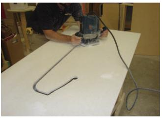
Use an overhang bit or trim bit with oversized nylon bearing to remove solid surface from inside of bowl.
