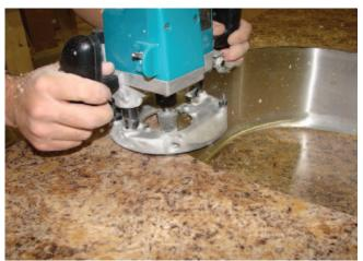
Trimming of the laminate back to the bowl wall should be done with a 10° bevel bit with an oversized bearing (bearing 1/8" oversized). Both Amana and Velepec stock Edge sink bowl bits.
