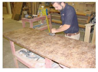
Roll laminate with a j-roller. Roll gently on rim of sink
