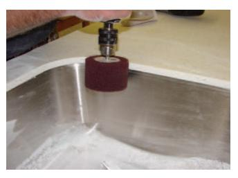
A non-woven flap wheel (available from Karran) works well for final buffing and finishing.
