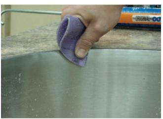
Final touch up of laminate edge if needed can be accomplished with a fine grit sandpaper. This also assists in removing scuffs and scratches that may have occurred during the sanding stage.
