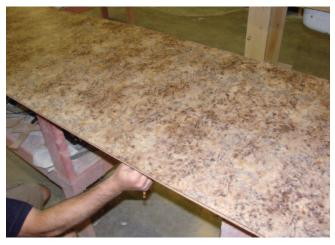
Place the laminate that has been cut to size (oversized by your shops standard amount) over the substrate. Trace the sink cutout in the substrate onto the back of the laminate.
