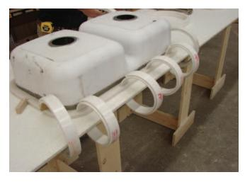
Place sink into marked position as indicated by the wood locator blocks. Use your preferred clamping method to clamp sink in place while adhesive cures for 30 to 45 minutes.
