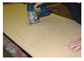
Using a jig saw make the cutout. When doing more than one sink of the same design, save time by making a wood template and using a router. Remember to reduce the size of the template by the thickness of the router bit to be used.
