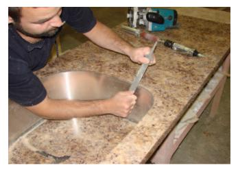
Removing the last remaining overhang of laminate and seaming adhesive may be accomplished by hand filing. Use an assortment of files included flat and round files to hand file the edge of the laminate until it is flush with the bowl wall.
