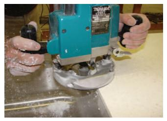
Trimming of the solid surface should be done with a 10° bevel bit with a 1/8" oversized nylon bearing. Adjust the height of the bit in the router until it is cutting as much of the solid surface away as possible without touching the sink. Pay close attention during this stage as setting the bit too low and touching the sink with the router bit may irreparably damage the sink.
