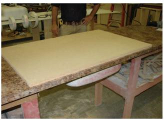
Place one or two sheets of particleboard over the sink area to provide even pressure while seam adhesive cures for approximately 30 minutes. The countertop should not be moved while adhesive is curing.
